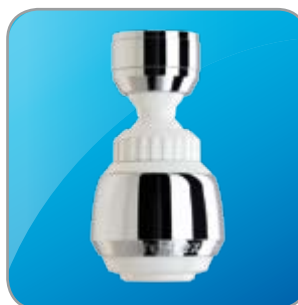
Ref. 2505/5OS aerator-shower CHROMED/WHITE with double brass swivel Threads: 22x1M female 24x1M male
