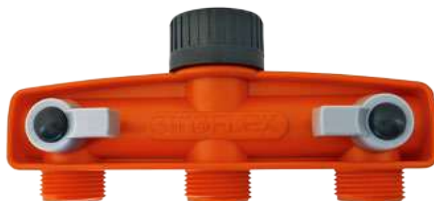
art. 4520 This 3 way manifold is provided with 3 individual taps and a 3/4" female cap which allows the plugging of the middle outlet. This unique design, which is compact and functional, provides the option of three separate and adjustable watering outlets in one unit.
